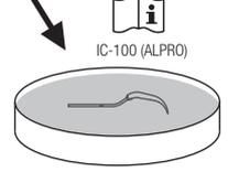
3  $\leq 38^{\circ}\text{C}$   $\geq 3.5 \text{ L/min}$   $\geq 30 \text{ sec.}$
